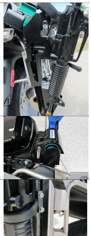
The gun lock release is actuated by the lower (unmarked) button on the RH "donut" switch cluster. The switch is active anytime the ignition is "ON" and for 30 seconds after ignition is turned "OFF".
