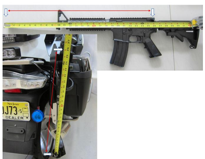
Insert the muzzle of the weapon in the muzzle cup and slide the barrel support up or down until the magazine just clears the upper side of the magazine opening.
