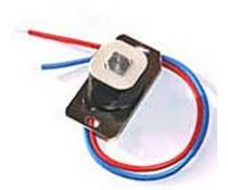
**LAPD Rear Gun Lock Release:** LAPD K52SF units are fitted with an additional release button at the rear of the motorcycle, together with an adjustable Gun Lock Timer via special request. Note that the terminals on the supplementary gun lock harness are specific to the LAPD rifle mount. Alternatively, a harness with the BMW terminals is available on the FMS Accessories website.
