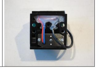
Drill a hole in turn signal housing and route wire directly inside to leave no exposed wire.
