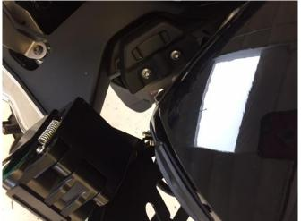
Remove the six bolts securing the radio box plate to the motorcycle frame. You do not need to remove the screws securing the lower trim panel to the radio box plate. **Note:** To remove forward screws, release the 8-pin helmet headset interface plug from the bracket to reach that screw.
